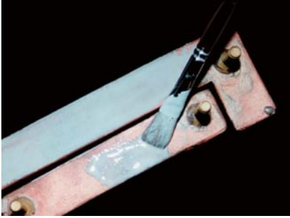
Cerabond™ 571 coats copper induction heater.
