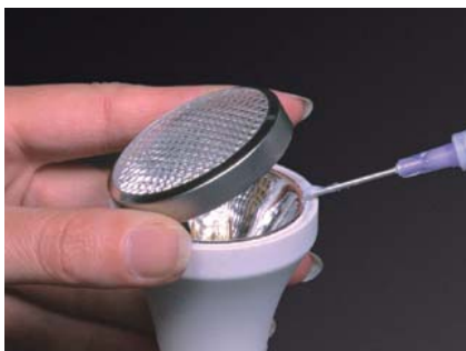
Cerabond™ 835-M bonds cover to halogen lamp.
