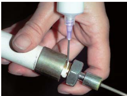
Cerabond™ 671 used as a high temp threadlocker.
