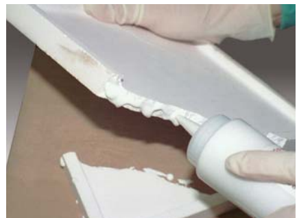
Cerabond™ 503 repairs furnace saggar plate.
