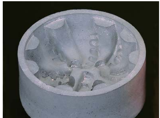
Ceramacast™ 673 mold for down-hole drill bit.
